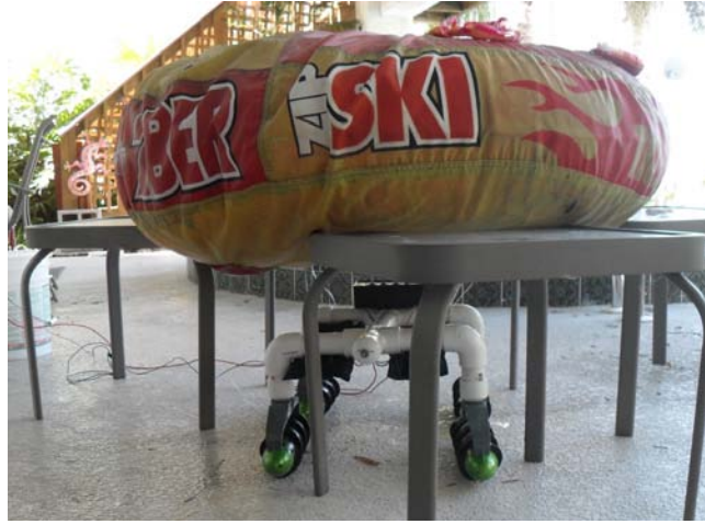
Figure 45: The inflatable tube used to suspend the test-bed.
