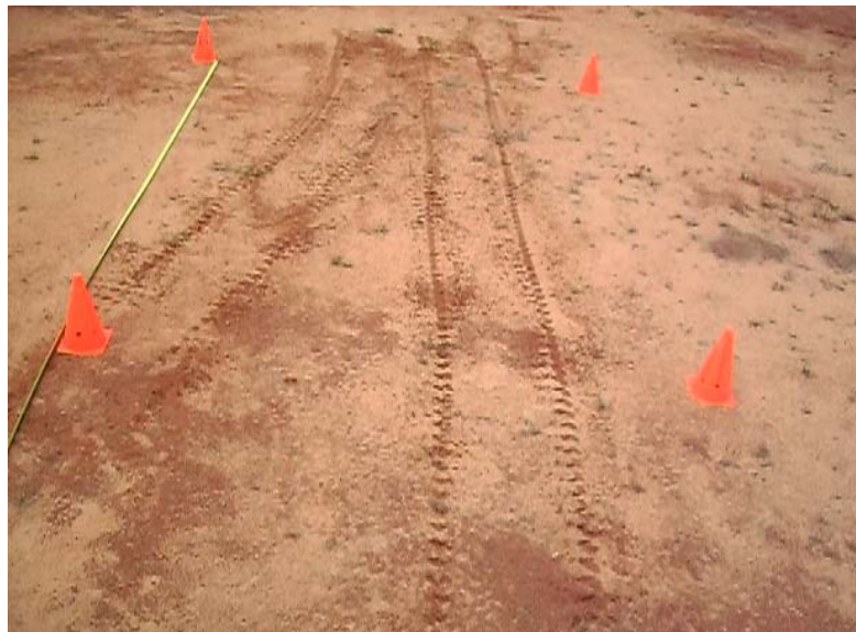
Figure 52: Inline-screw tracks in clay. The tracks were from longitudinal tests.
