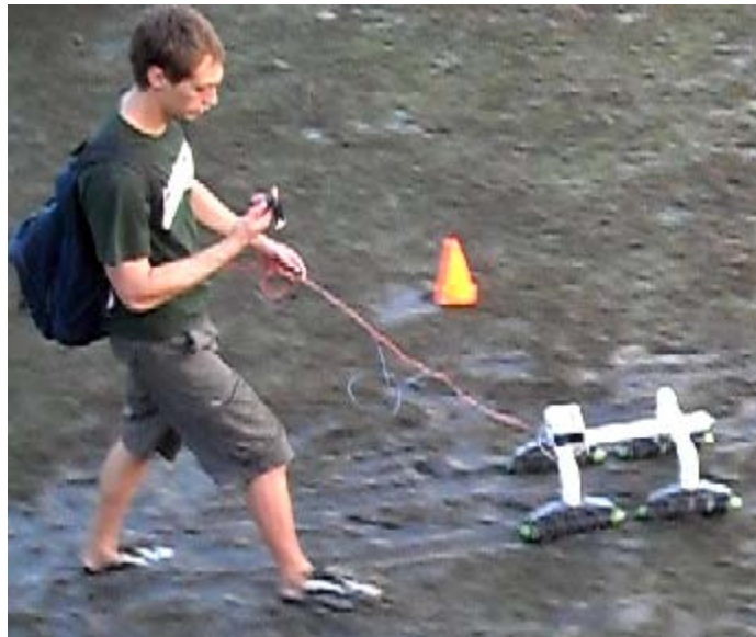
Figure 43: The author shown alongside the test-bed. A motorcycle battery in a backpack is utilized to power the test-bed.
