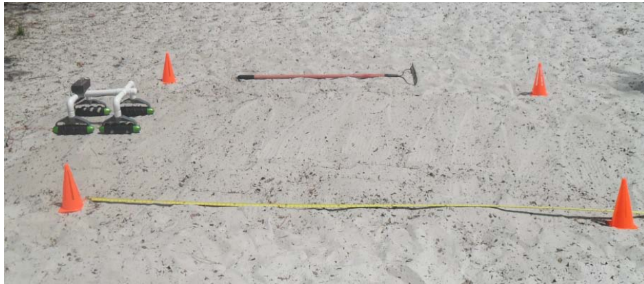
Figure 50: Sand terrain test setup. The rake used to flatten the sand is shown.
