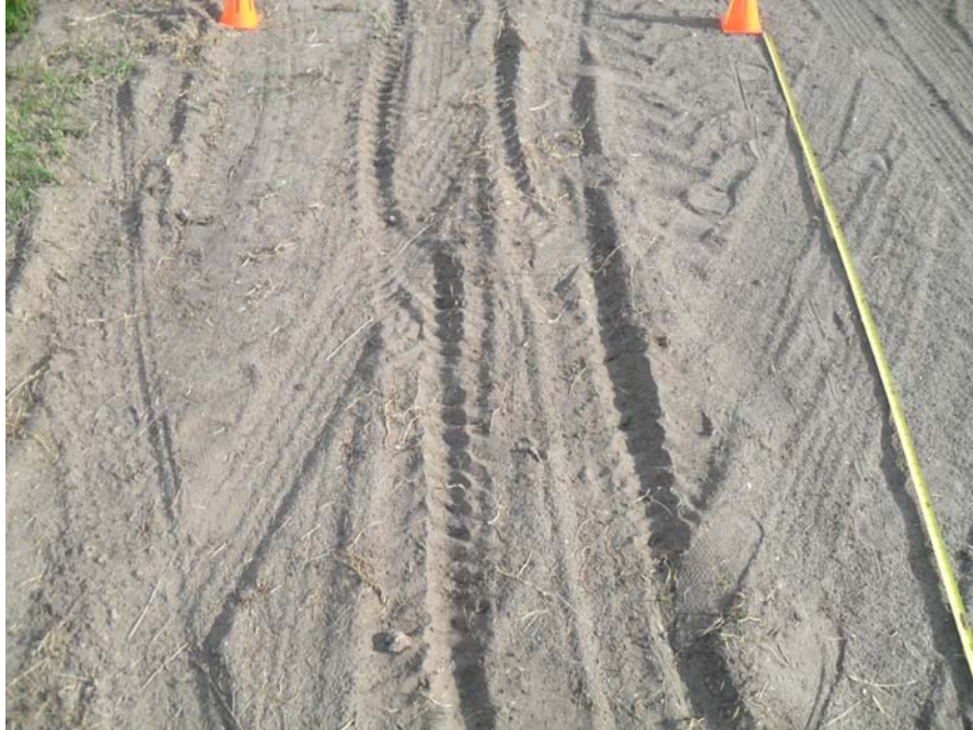
Figure 48: Tracks from the inline-screw deviating in dirt.
