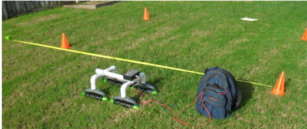
Figure 47: Test setup for grass terrain.
